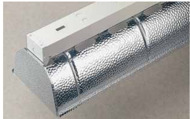
With the upright grooves directional air circulation is created, which prevents disruptive dust deposits on the reflector.
