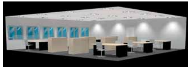
Office with U7 luminaires. Walls: \bar{E}_m = 241 lx and U_o = 0,38 Ceiling: \bar{E}_m = 141 and U_o = 0,55
